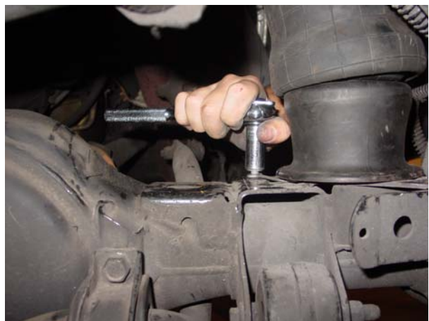
6. Remove the bolt securing the lower air spring retaining pin to the front axle. ↑
