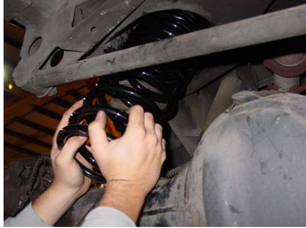
8. Install coil spring onto rear suspension. ↑ Align the upper aluminum spring mount in place.
